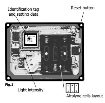
If necessary, adjust light intensity of the lcd display.
