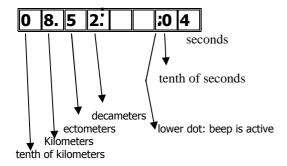
The first 4 digits on the left of the display show the theoretical distance from start (precision:10 meters). The two digits on the right side of the display show the countdown in seconds to the next 100 meters.
